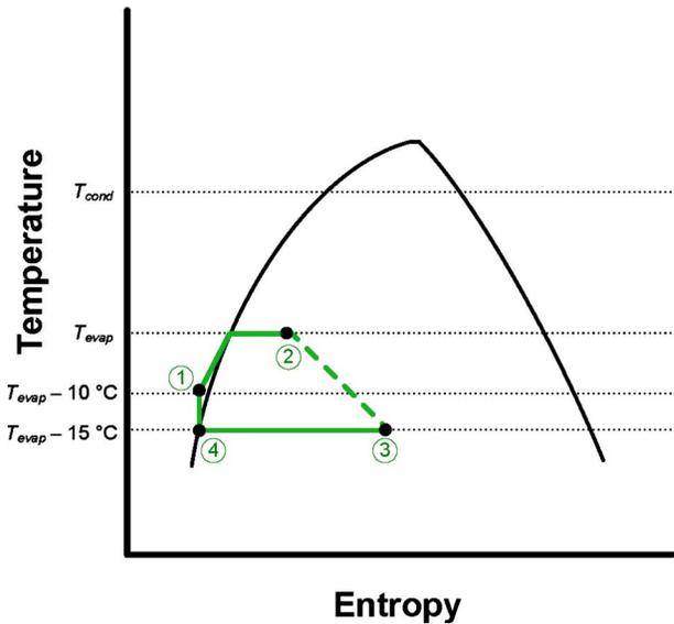
Fig. 6  $T$ - $s$  (temperature-entropy) diagram for cycle 3 (pumped loop with thermoelectric cooler)
