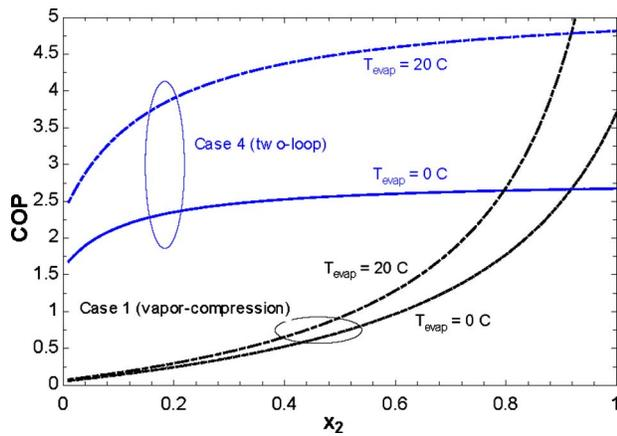
**Fig. 9 Comparison of the single-loop (case 1) and two-loop (case 4) configurations based on COP for two different evaporator temperatures ( $T_{\text{cond}}=40^{\circ}\text{C}$ )**
