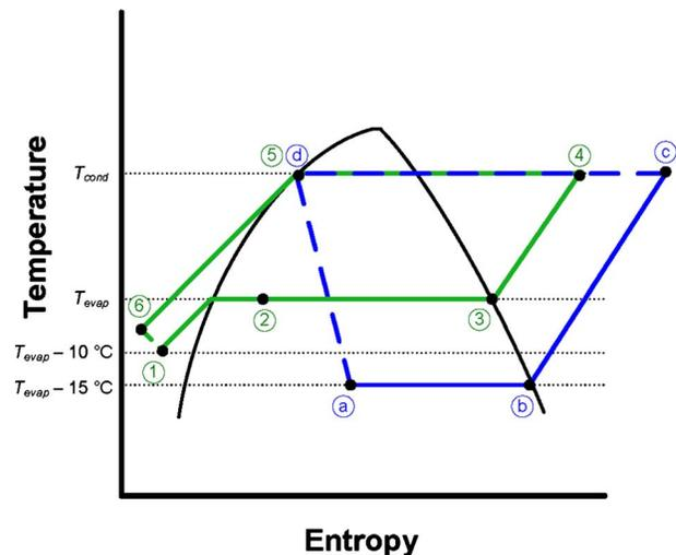
Fig. 2  $T$ - $s$  (temperature-entropy) diagram for cycle 1 (conventional vapor-compression cycle cascaded with a second vapor-compression cycle)
