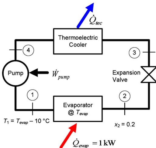
Fig. 5 Schematic diagram of a pumped-loop system cooled by a thermoelectric cooler (cycle 3)
