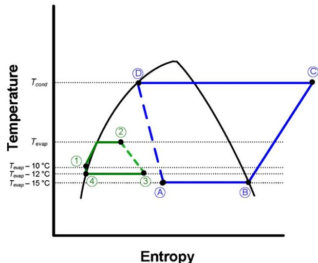
Fig. 8  $T$ - $s$  (temperature-entropy) diagram for cycle 4 (two-loop system)
