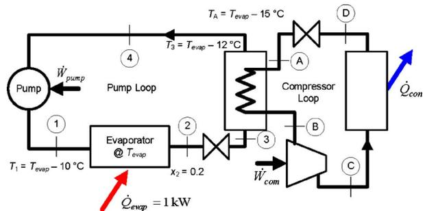
Fig. 7 Schematic diagram of a two-loop system (cycle 4)
