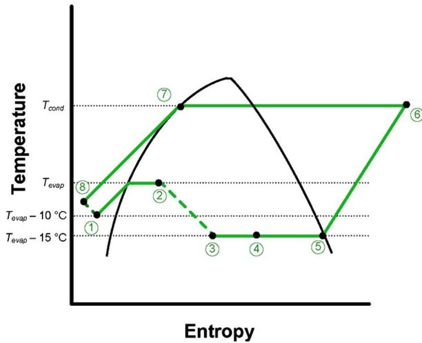
Fig. 4  $T$ - $s$  (temperature-entropy) diagram for cycle 2 (conventional vapor-compression cycle with an economizer heat exchanger)
