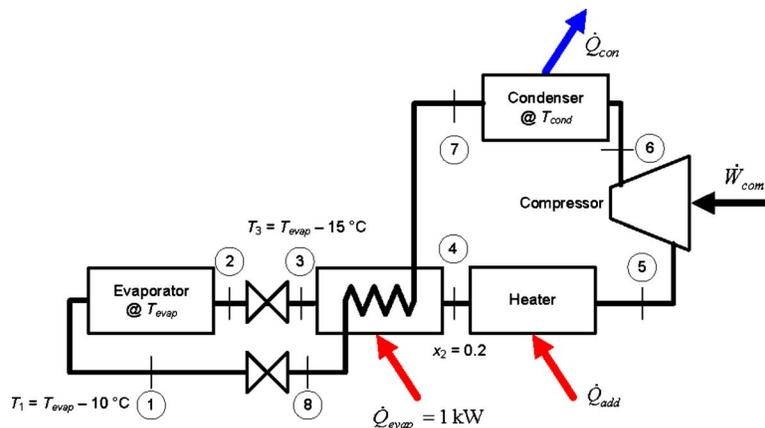
**Fig. 3 Schematic diagram of a vapor-compression refrigeration system with economizer (cycle 2)**
