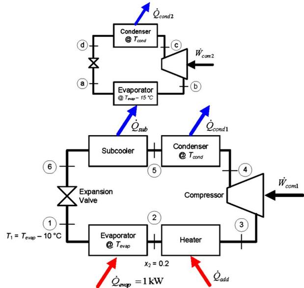
Fig. 1 Schematic diagram of a conventional vapor-compression refrigeration system (cycle 1), with a second vapor-compression cycle cascaded to produce subcooled conditions at the evaporator inlet
